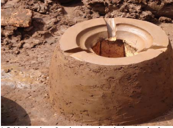
A finished product of rural stove ready to dry in a couple of days
